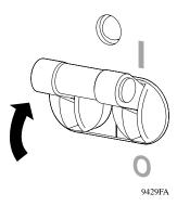
10. Turn the power supply switch to the on position.
